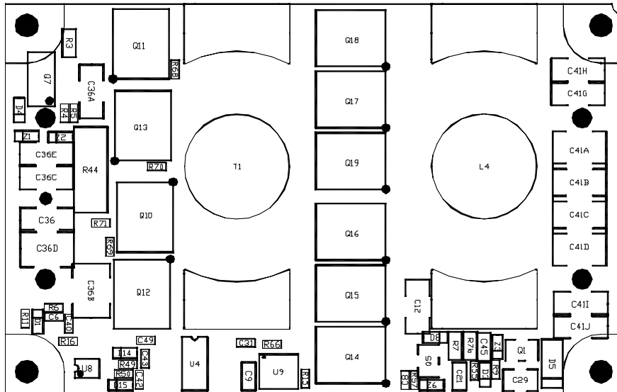
Layout of components on top side
