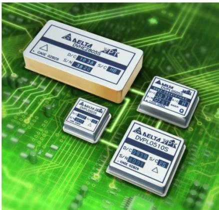
With the new variety of POLs available with current ratings of 3A, 5A, and 10A that meet MIL-PRF-38534 and MIL-STD-883, today's commercial avionics, military and space systems designers have smarter, newer options in designing high performance systems that meet evolving light weight, high performance, and low cost system requirements.
