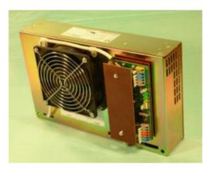
Fuses: F1 (connected in L+): 20A/250V, F2 (connected in B+): 20A//32V (automotive type)
