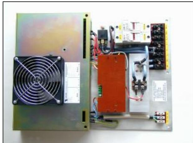
**Fuses: F1 (connected in L+), F2 (connected in B+), value 50A**
